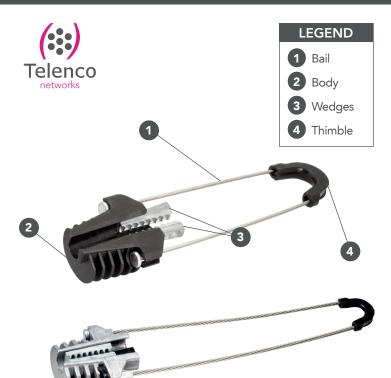
Telenco® Acx BGB clamps are used for the deadending of aerial figure-8 cables or aerial figure-8 duct structures with steel messenger on access networks where spans do not exceed 90m. They are particularly recommended for installation in Northern countries characterised by harsh climate conditions.
